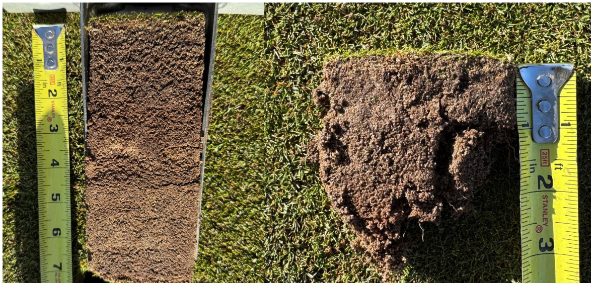
A profile collected from No. 15 Vistas shows a rootzone with good drainage properties and no soil layering that would prohibit root development (left). On the right, a close-up image shows a healthy mixture of sand and organic matter at the surface.
