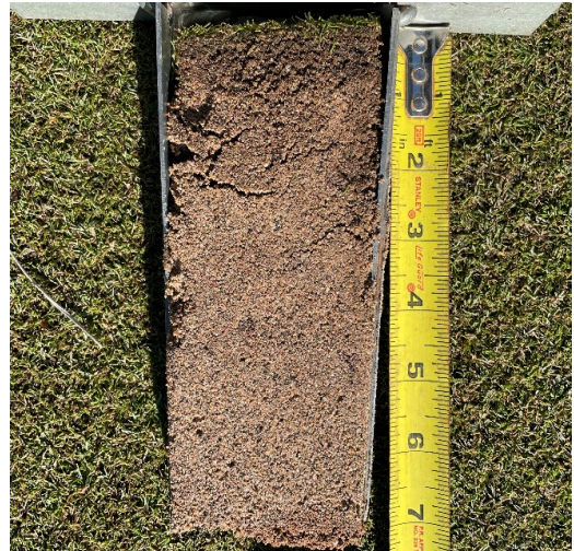
There is no indication of excessive organic matter within the top 1 inch of the practice putting green.
