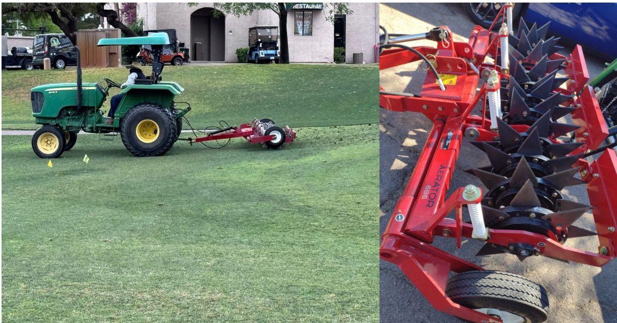
A tow-behind slicing tool is effective to encourage water infiltration and improve bermudagrass recovery. This tool is inexpensive, reliable and fast.
